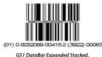
GS1 DataBar Expanded Stacked.
